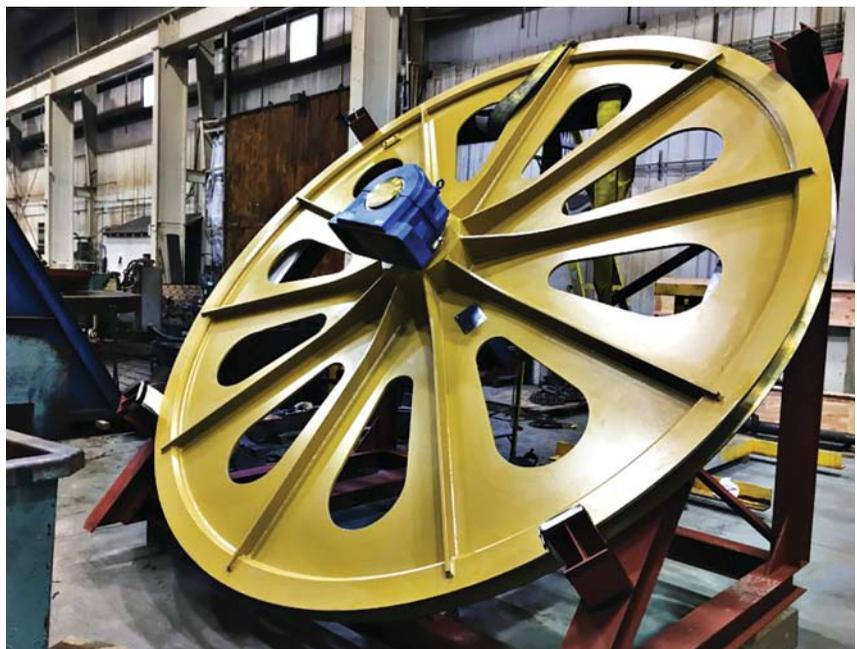
NMT's gold head sheave, above, can be designed split for ease of transportation and installation. (Photo: NMT)
