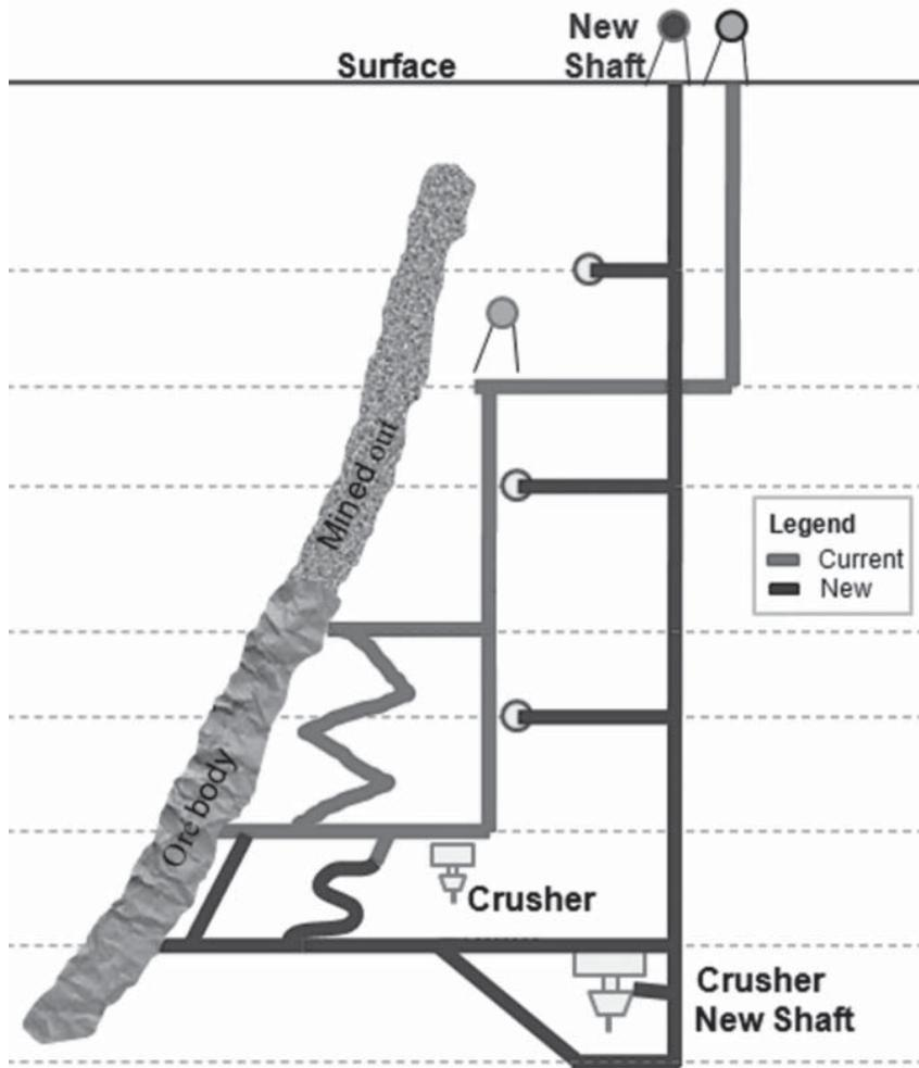
A mining flow diagram for both mines at the Mopani Deeps Project in Zambia. (Image: FLSmidth)
