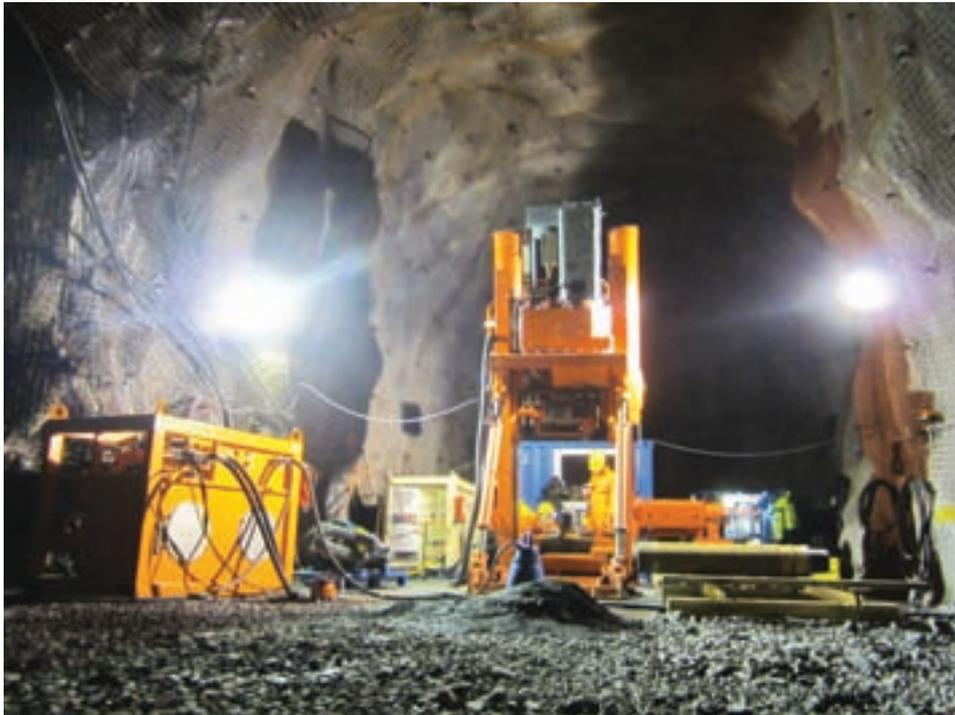
**A mid-sized RHINO raise borer at a drill site** ► In raise boring the risk of rock falls and the handling of explosives is eliminated as the operation is mechanised. The final product of the method is a raise excavated with minimal disturbances to surrounding rock. "This is advantageous in ore
