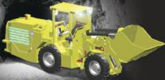
movement. There is no need for a cable reel, enhancing the reliability of the machine. Plus, there is the saving of the expensive cable. Aramine's new engine technology using battery power "allows a general structure without hydrostatic system, this also improves the reliability of the machine," the company says.
