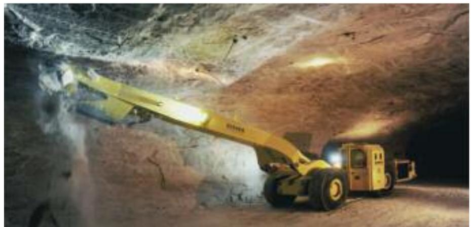
*A larger version of this upgraded GHH LF-7HB shearing scaler (shown here) is based on the new LF-21H with a maximum permissible scaling height of 11 m and will be available soon*
