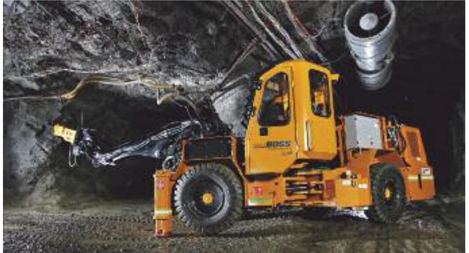
sophisticated battery management and vehicle monitoring capabilities, as well as onboard charging that ensures compatibility with existing mine infrastructure.
