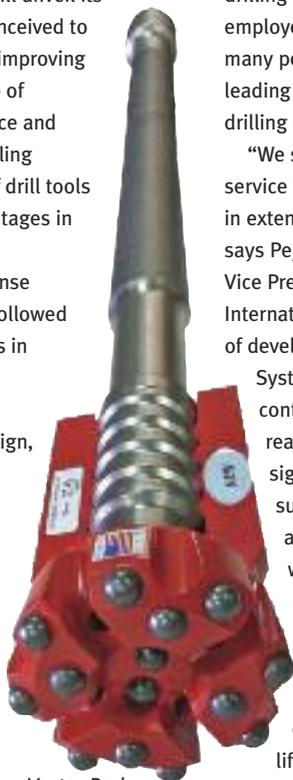
*Rockmore International's new Vector Rod System is offered in multiple configurations of button bits, MF rods, and shank adapters. These drill string components are available in XT38, XT45, XT51, and XT60 thread types, designed to improve drilling productivity and reduce extension drilling operating costs in surface and underground percussive drilling*
